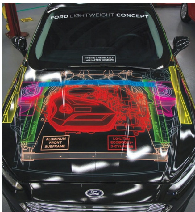
An aluminum front subframe and a chemically laminated windshield are just some of the innovations in Ford's Lightweight Concept vehicle. Image courtesy of Ford Motor Co.
