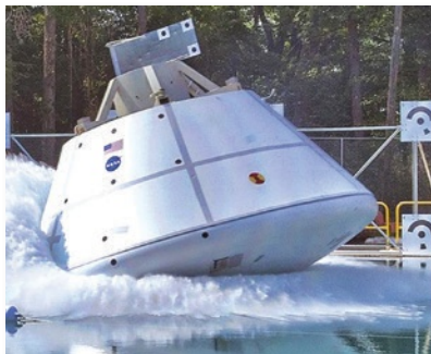
Orion Multi-Purpose Crew Vehicle splashdown test (left) and software simulation of loads on the vehicle (right). Images courtesy of NASA and Collier Research Corp.
