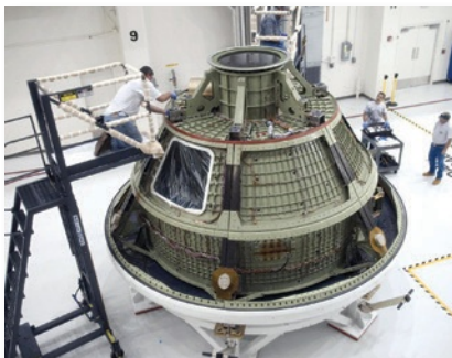
The Orion Ground Test Vehicle at NASA's Kennedy Space Center. The circular heat shield is visible at the base of the vehicle. Image courtesy of NASA and Collier Research Corp.
