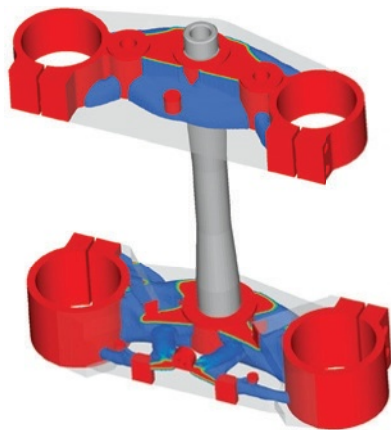
Topology optimization results with manufacturing constraints applied.
