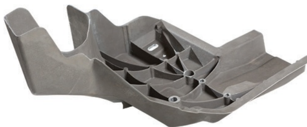
The kickdown casting used in the Ford Lightweight Concept vehicle reduces weight by incorporating many stampings in the foot pedal region of the body in white structure. Image courtesy of Cosma International/Magna International.
